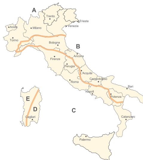
Fig. 3: Suddivisione del territorio nazionale in zone climatiche (circa. Min. LL.PP. n. 22631 del 24. 05. 82. Fig. 3: Division of the Italian national territory into climate zones (Min. Public Works, circular no. 22631 of 24. 05. 82).
